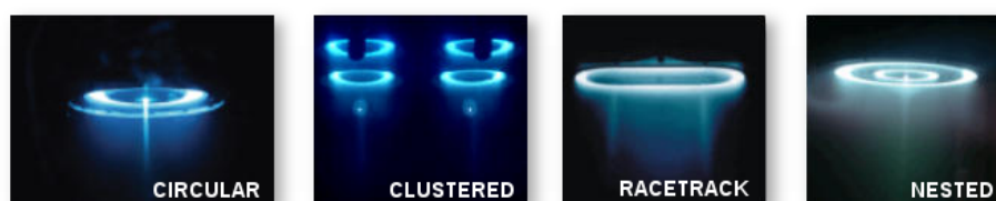
Figure 1.4: Busek multiple cluster configurations [1]
